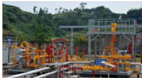
On-line sour gas corrosion test unit max. pressure 35MPa, max. temperature 80°C
